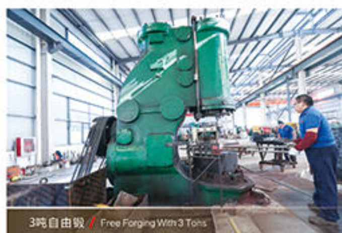
3吨自由锻 / Free Forging With 3 Tons
